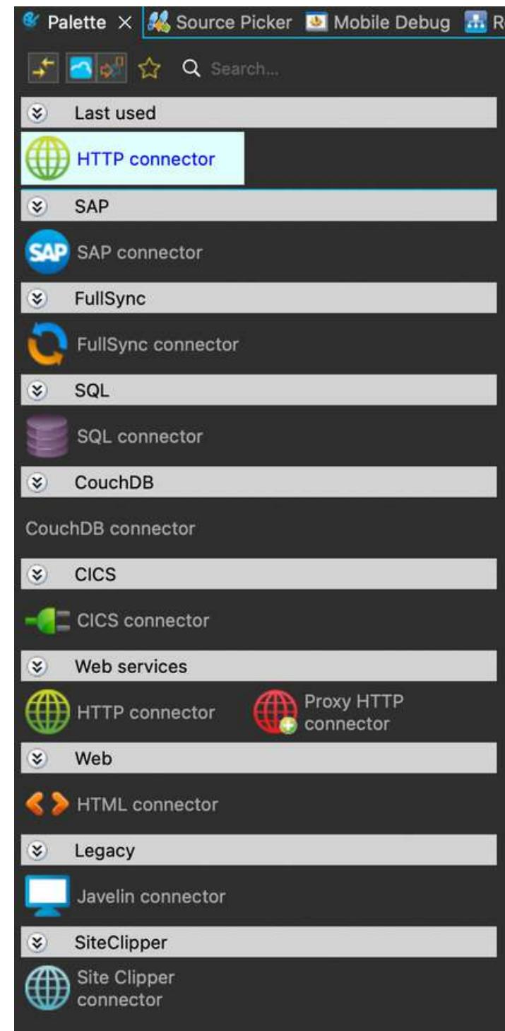
There are **different connectors and transactions** in Convertigo, used for **different data providers** (SQL, Web services, Legacy apps running on mainframes...).
